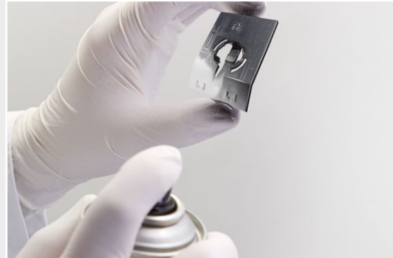
2. Painting of the blank with LPKF ProtoPaint LDS
