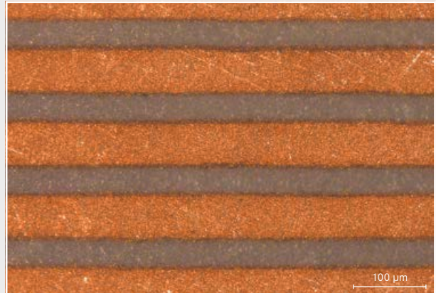
High-precision structuring of metal layers on ceramics
