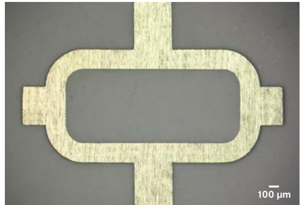
Minimum thermal impact on FR4 material
